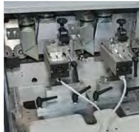
Milling unit before bending rollers
